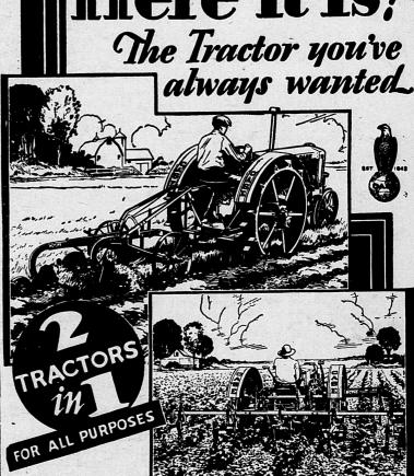
ERE, in the new Model "CC" Case, is a tractor that successfully combines a plowing and a cultivating tractor in one machine. It is the first tractor to offer a variable wheel spacing feature by which the rear wheels can be easily moved in or out, from standard 48-inch tread for plowing to various treads, up to 84 inches, for row crop planting and cultivating. This is the tractor you've always wanted. It fits all
